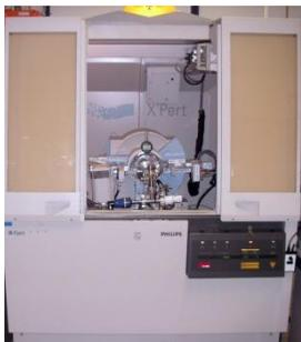
Fig.3.10(a) X'Pert pro Multipurpose Diffractometer (MPD)
