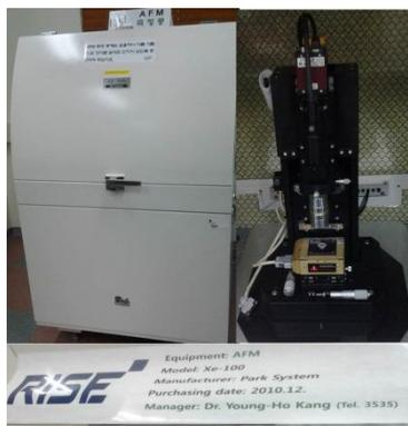
Fig. 3.6 Atomic force microscope (AFM)
