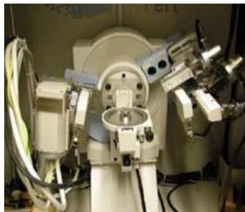
Fig.3.10(b) XPERT XRD with X'celerator Detector for thin film
