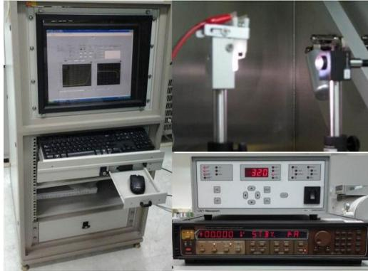
Fig. 3.13 AM 1.5 solar simulator system
