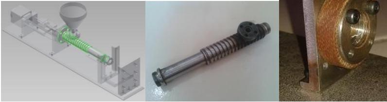
**Figure 13 CAD Drawing and Manufactured Products of Injector Barrel and Flange**
