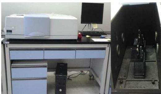
Fig.3.1 Lambda 750 UV/Vis/NIR Spectrophotometer
